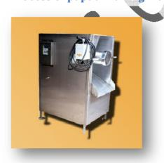
**Dough mixer (floor kneading machine):** this machine would consist of heavy-duty stainless steel body with multi-purpose arms. Heavy-duty gears are providing to take the full load and to avoid damage to the mixer arms.
